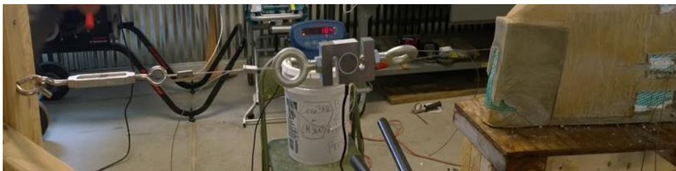
Figure 19: Post-Tensioning with Inline Force Gauge
